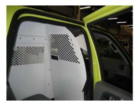
Attach "B" pillar mounting bracket to front partition using 1/4" x 3/4" carriage bolts and nuts
